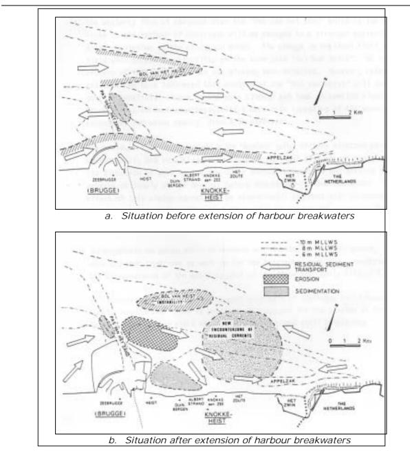
Fig. 4: Changing of current, sedimentation and erosion pattern due to extension of harbour breakwaters.
