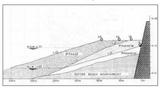
Fig. 7: Cross section of nourished beach at Knokke-Heist.
