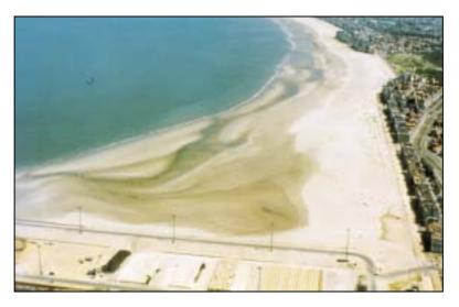
Fig. 9: Nourishment directly downstream of harbour breakwater.
