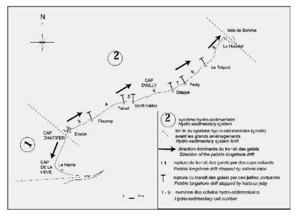
Fig. 2 : Direction of the longshore transport and the hydro-sedimentary cells (Costa, 1997).
