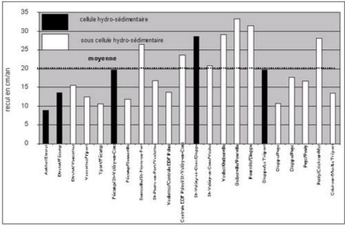
*Fig.9: Haute-Normandy cliff erosion by hydrosedimentary cells between 1966 and 1995 (Costa, 2000 in CPIBP).*
