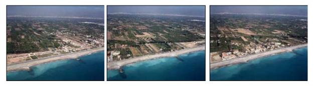
Figs. 12, 13 & 14: Different views of the set of groins built on La Torre beach.
