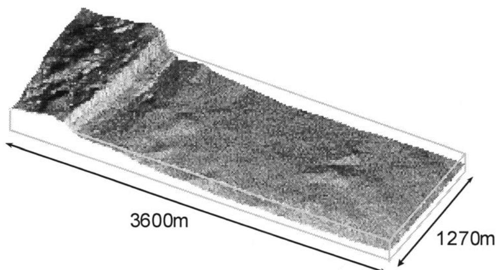
**Fig. 2.** Shaded perspective view of a DTM for a section of the coast near Easington.
