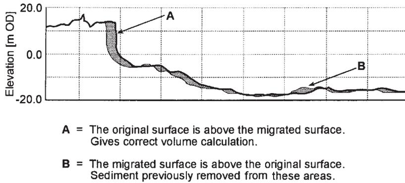
**Fig. 3.** Horizontal section through the original DTM. The change after lateral migration is indicated by the cross-hatched area, which represents the volume of sediment yielded.
