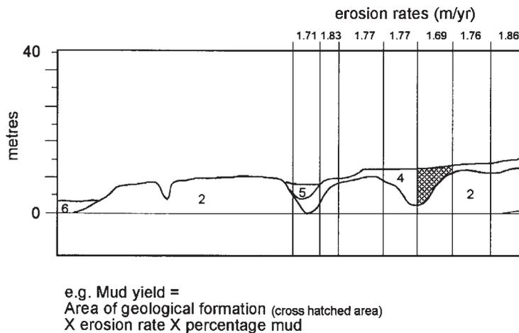
**Fig. 4.** Horizontal geological section used to calculate the sediment yield by lithology.
